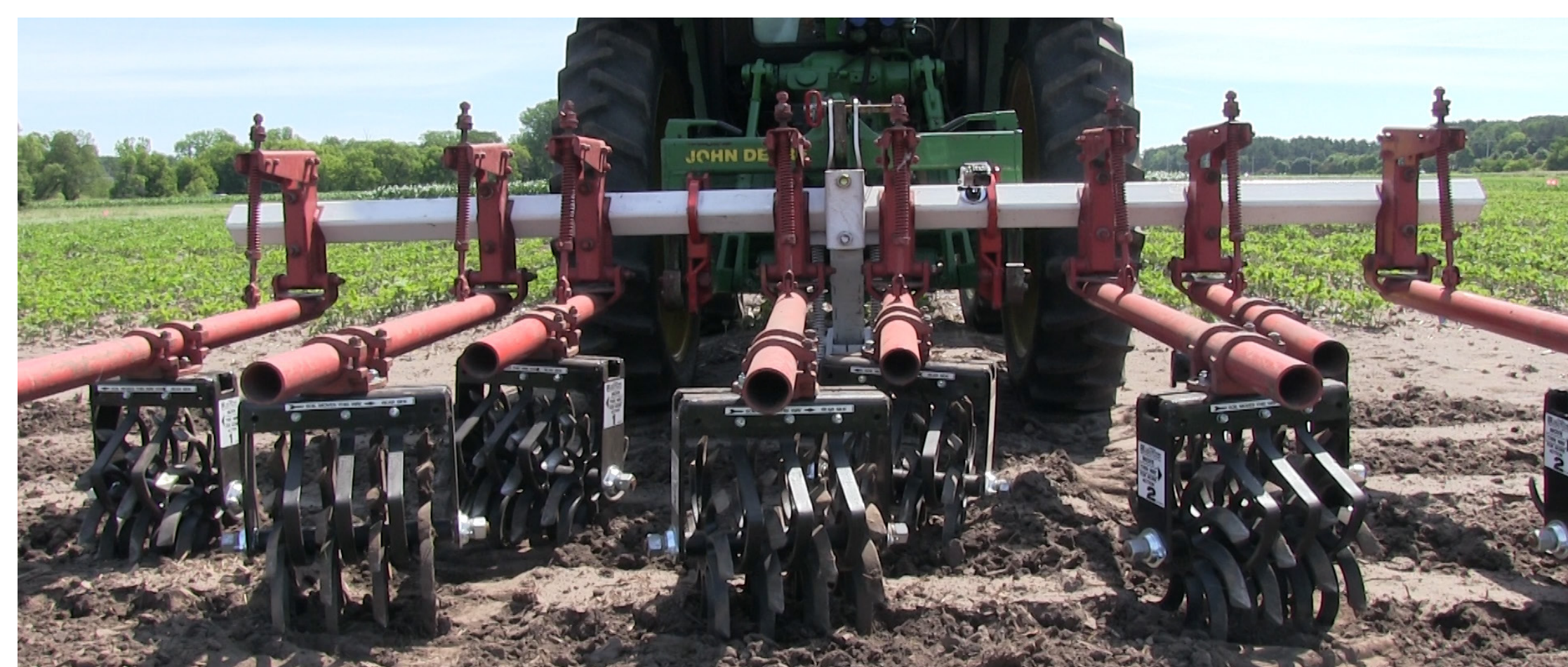
Figure A. Lilliston cultivator used to incorporate cover crop seed 6 days after POST. Cultivator ran at 7-8 MPH and set to move soil away from corn plants.
