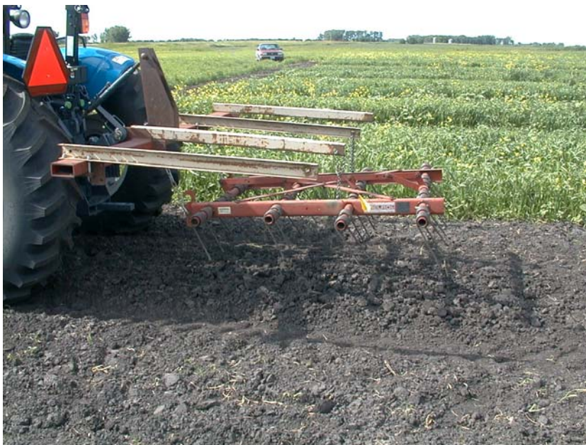
4-bar spring tooth harrow used for the weed control study
